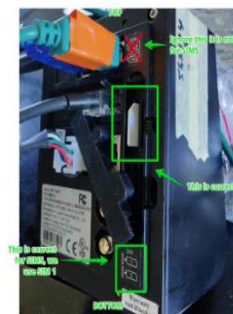
Above: Full Size LYNK, with the SIM card inserted in the upper left SIM card slot, with the notched corner facing up.
