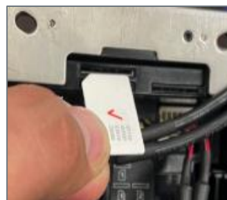
Above: An Overlay LYNK with the SIM card inserted in the upper left SIM card slot with the notched corner of the card facing up.
